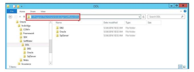
For SQL Server, new backup files are included in the Insbridge download in the Windows folder under databases. If the IBSR backup files cannot be used and DDL scripts are needed, SQL Server DDL scripts can be found on the server where Insbridge was installed in the .../Oracle/Insbridge/SoftRater folder.
